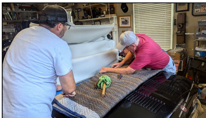
Tim McMurray and Kenny Widner install the convertible top trim.
