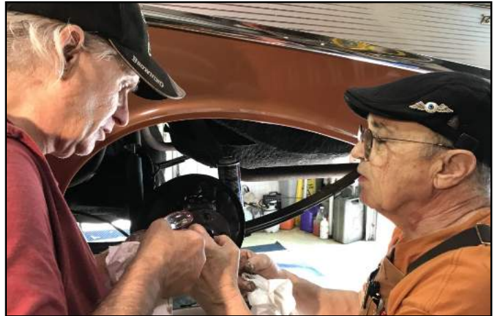
Stan and Dan inspect brake parts under a magnifying glass to determine which ones can be re-used.
